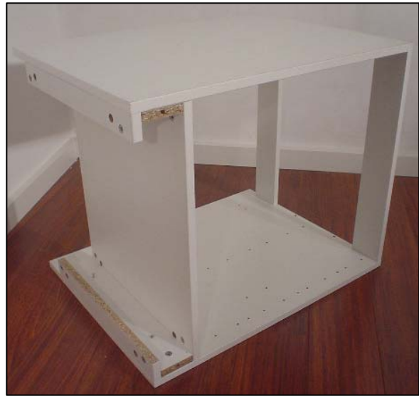
11.2. Fit remaining Support Rail
